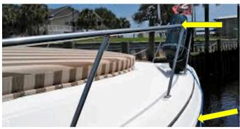
If your cruisers railing is recessed more than 4" relative to the Rub rail, please add the provided spacer. The spacer allows installation closer to the rub rail by extending the Power Fender out from the railing. Add the spacer between the Power Fender and the clamp:
