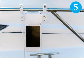
If the boat has a lifeline, it should be placed under or behind the Power Fender. Make sure the lifeline doesn't interfere with the fender's movement. The lifeline should not be too tight, as when temperatures drop it will get tighter and may damage the Power Fender's enclosure.
