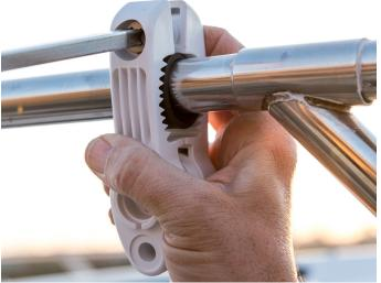
Install the Power Fender in front of the stanchion (to the left of the stanchion). Lightly tighten the bolts to allow clamp movement along the railing during the installation:
