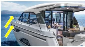
But in some cruisers the railing is significantly recessed relative to the Rub rail:
