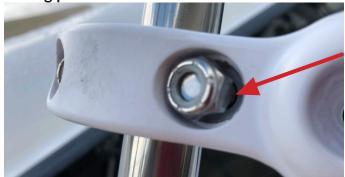
Nut is not fully inserted.
