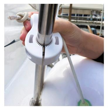
Pull the line firmly while holding the front clamp, and confirm that the knot doesn't slip out through the clamp hole. The first installation stage is complete:
