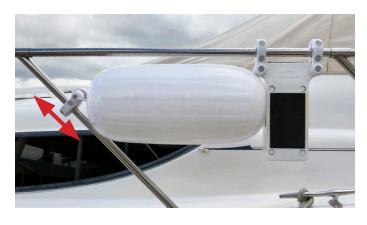
While the fender is touching the Power Fender; the distance between the fender to the front clamp and the Stanchion should be 1/2". Move the Power Fender along the railing to achieve the desired location:
