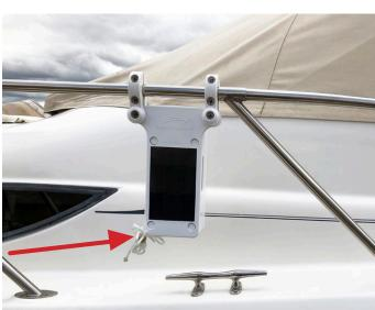
Remove the rubber band from the Automatic Fender line and run it through the fender's center hole:
