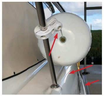
Move the front clamp up or down the Stanchion until the fender is parallel to the railing:
