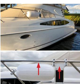
Connect a clamp to the Automatic Fender using a single bolt and a single nut. **Lightly** tighten the bolt.
