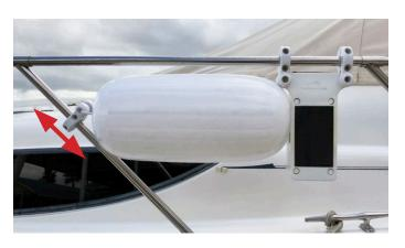
While the fender is touching the Automatic Fender; the distance between the fender to the front clamp and the Stanchion should be about 1/2". Move the Automatic Fender along the railing to achieve the desired location:
