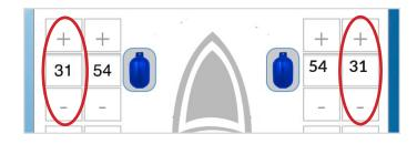
Press "**Rub Rail**" again to test the new line length. Repeat these steps until the desired rub rail line length has been achieved.
