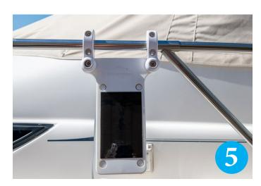
If the boat has a lifeline, it should be placed under or behind the Automatic Fender. Make sure the lifeline doesn't interfere with the fender's movement. The lifeline should not be too tight, as when temperatures drop it will get tighter and may damage the Automatic Fender's enclosure.
