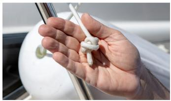
Pull the line firmly while holding the front clamp, and confirm that the knot doesn't slip out through the clamp hole. The first installation stage is complete:
