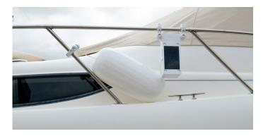
Install the Starboard Automatic Fender in the same manner.
