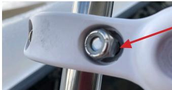
Nut is not fully inserted.
