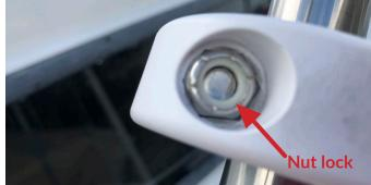
**Note:** The nut lock is to the outside. The nut is fully inserted into the plastic groove.
