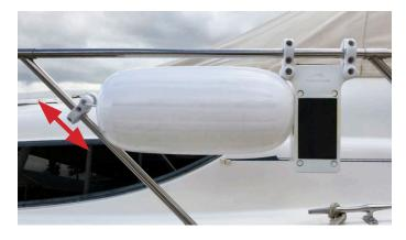
While the fender is touching the Automatic Fender; the distance between the fender to the front clamp and the Stanchion should be about 1/2". Move the Automatic Fender along the railing to achieve the desired location:
