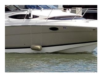
You can always change them back to vertical deployment by lifting and deploying again. If docked in choppy water, hang your manual bow fenders and lift the Automatic Fenders to rail level. While docked, hanging the manual fenders is usually easily done from the dock.
