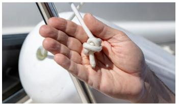
Pull the line firmly while holding the front clamp, and confirm that the knot doesn't slip out through the clamp hole. The first installation stage is complete:
