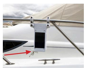
Remove the rubber band from the Automatic Fender line and run it through the fender's center hole:
